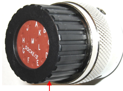
Remove the thread protector
